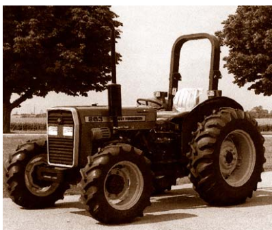
Massey Ferguson 263 - 8 Speed Manual Trans. 40km/h 4 RM/WD OCDE/OECD 2/1850
