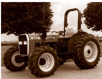
Massey Ferguson 243 - 8 Speed Manual Trans. 40km/h 4 RM/WD OCDE/OECD 2/1849
